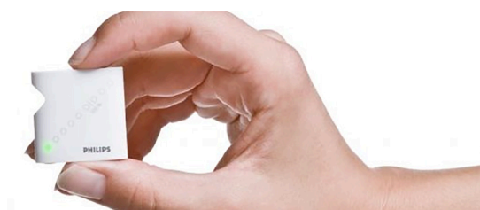
Figure 8. DirectLife activity monitor or accelerometer Tracmor D .
